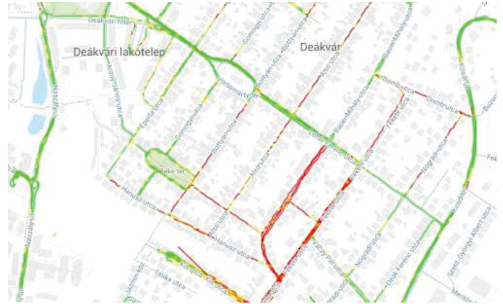
Fig 1: Road surface data collected by Route4U users. Legend: red - very rough surface (such as cobblestone); yellow and orange - intermediate roughness (badly laid concrete plates, bad road quality); green - smooth surface (good quality asphalt)
